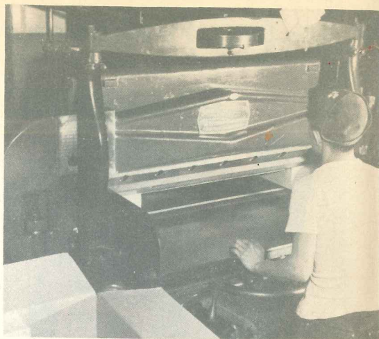
Power driven cutters easily handle sheet sizes up to 51" within hairline preciseness.
